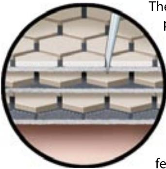
The technology works by “trapping and blocking” the needle. Most needles strike a guard plate directly, resulting in the immediate arrest of the needle. If the needle hits a gap, it is “trapped” and then blocked by the layer below. The gaps provide the flexibility required to allow the material to bend and flex.
